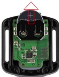
4. Install the new battery, keeping the “+” pole facing up.
