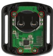
3. Lift the PCB board and slide out the battery, as shown in the picture.
