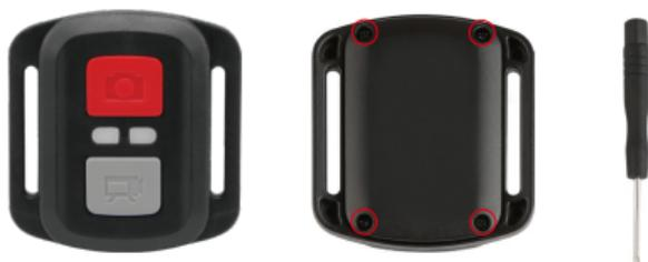
2. Remove the other four screws in the PCB board.
