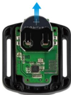
**Note:** Avoid rotating the circuit board to prevent reversing the remote control buttons.
