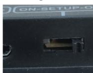
Slide the mode switch of the Wildlife Camera to the SETUP position to start the test mode. In the Photo or Video mode press the MENU button to call up the menu.
