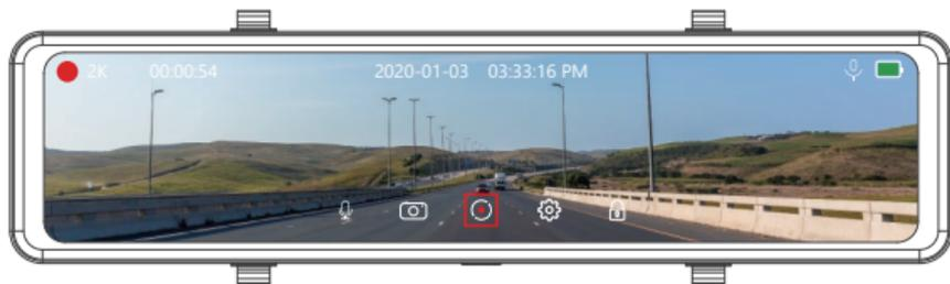
The time displayed in the top-left corner indicates how long has been recorded. When the time displays "0:00:00", that means the card is full. If turning on "Loop Record", you don't need to change or format the card, it still records and the latest file will automatically overwrite the existed file.
