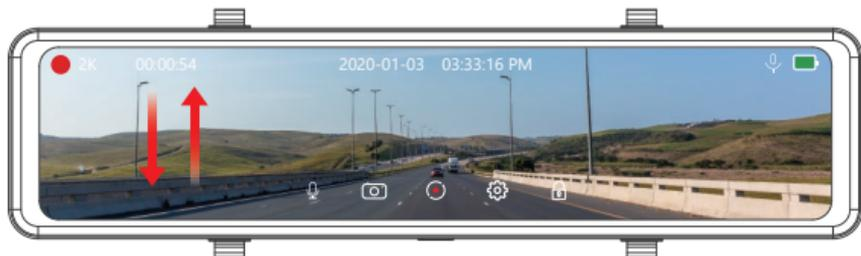
On the right screen, slide up or down by finger to adjust the screen brightness.
