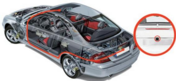
To use the reversing function, install the rear camera in position 2, then connect the red trigger cable of rear camera extension cable to the positive lead of the car reversing lamp.
