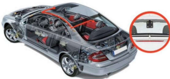
**Position 2:** Install the rear camera near the license plate. Position 2 is highly recommended. The back image is crisp and clear for both rear viewing and reversing guide.
